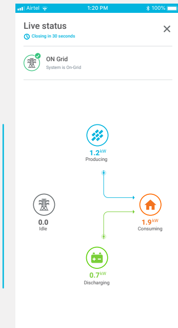
Solar production and battery discharge are powering the home.
