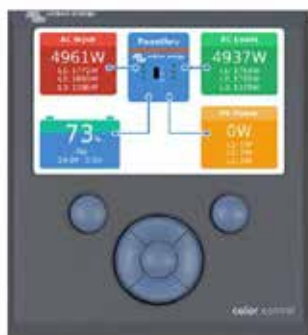
Color Control GX, showing a PV application
