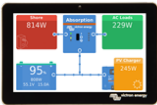
GX Touch (optional display for Cerbo GX)
