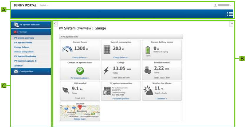
Figure 1: User interface of Sunny Portal (example)
