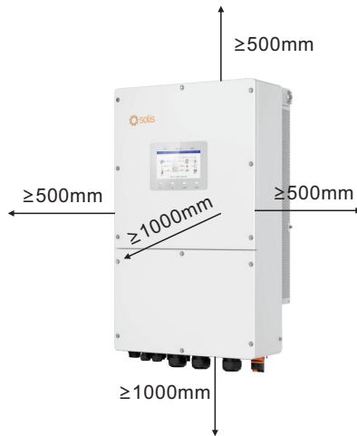
Figure 3.5 Inverter Mounting Clearances
