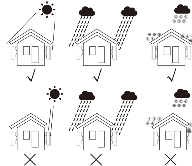
Figure 5.1 Recommended Installation locations
