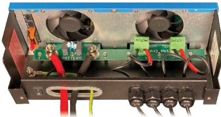
Inside the SmartSolar MPPT RS 450|100
