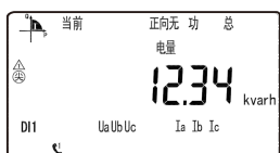
Current forward reactive energy 12.34kWh
