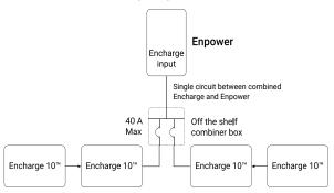
⚠ WARNING! Parallel power production sources only. Do not connect load circuits.
