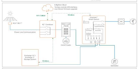
Partial home backup with main load panel as service entrance and PV combiner connected to Enpower.
