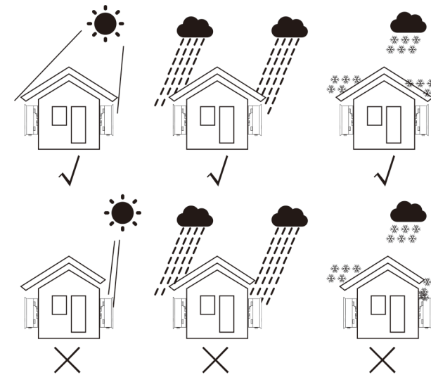
Figure 4.1 Recommended Installation locations
