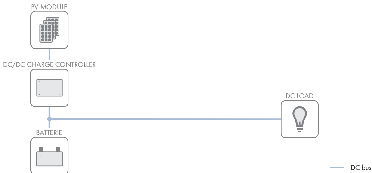
Figure 2: Example of a DC coupled system
